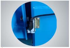
The safety stop device at the height of 300mm with tone alarm for safety.
