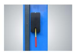
A manual locking safety release device controls the double locks.
