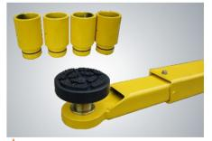
Features insert and screw rubber pads.
