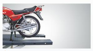
Rear Tire removal cover removable platform cover plate is convenient for rear wheel changing.
